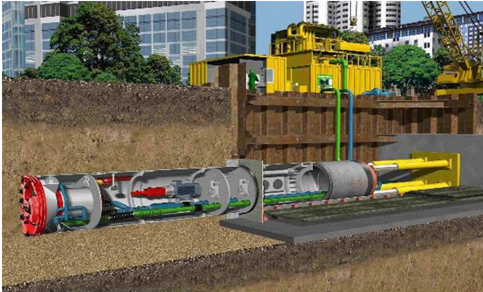
Plate 3.10: Indicative micro-tunnelling schematic
